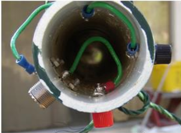
Fig 5. Binding Posts & Internal Wiring
